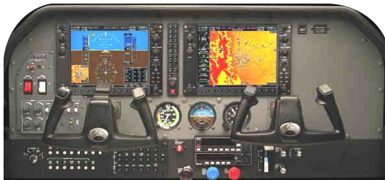
Cessna 182 Panel with Garmin G1000 display units
